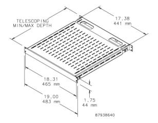
An easy-to-install tool-less vented 19-in. shelf. Mounts onto rack angles that have EIA-spaced square holes (.375 in.). Shelf slides open and provides a variable-sized, continuous surface for equipment. Back of shelf has oval cutouts for power and data cables. Accessory hole patterns at back of shelf fit small and large D-rings to help manage cable. Made of steel with a 150 lb. (68 kg) static load rating. Available with RAL 9005 black or RAL 7035 gray polyester powder coat finish.
